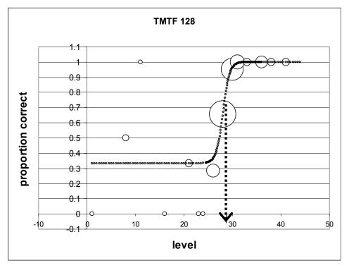
Sketch a sigmoid (Sshaped) curve by eye to data the points, weighting larger symbols more. Towards the left-hand side, your function should flatten out at chance level  $(\frac{1}{3})$ because you used Triples 3AFC format. Here's an example at left, with a threshold of about 28:
